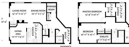
MAIN FLOOR PLAN Ceiling Height: 8'-0"
